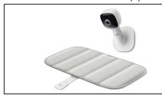
The EUT is a Video Baby Monitor system which consists of a Camera unit, Smart Sensor and Sensor Mat, the camera unit supports 2.4GHz FHSS and Wi-
